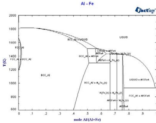
Figure 1. Phase diagram of Al-Fe system.
