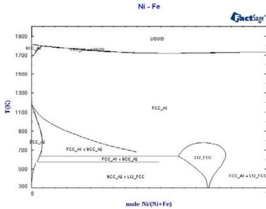
Figure 3. Phase diagram of Ni-Fe system.
