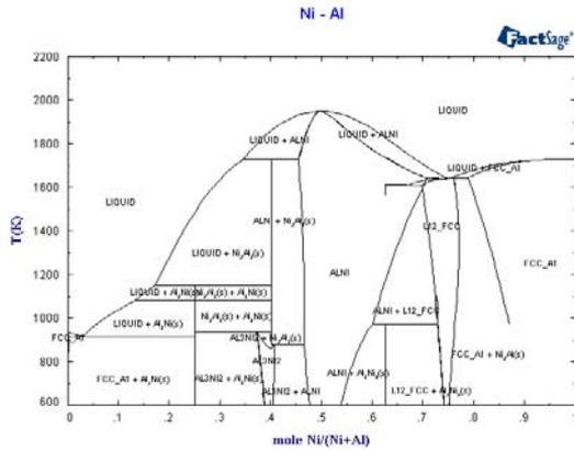
Figure 2. Phase diagram of Ni-Al system.
