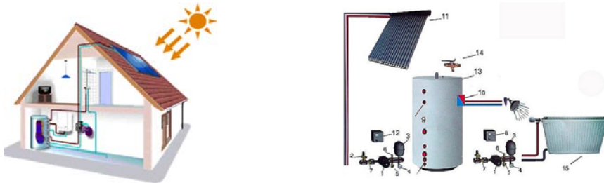
Figure 1. The use of solar collectors for heating and hot water
