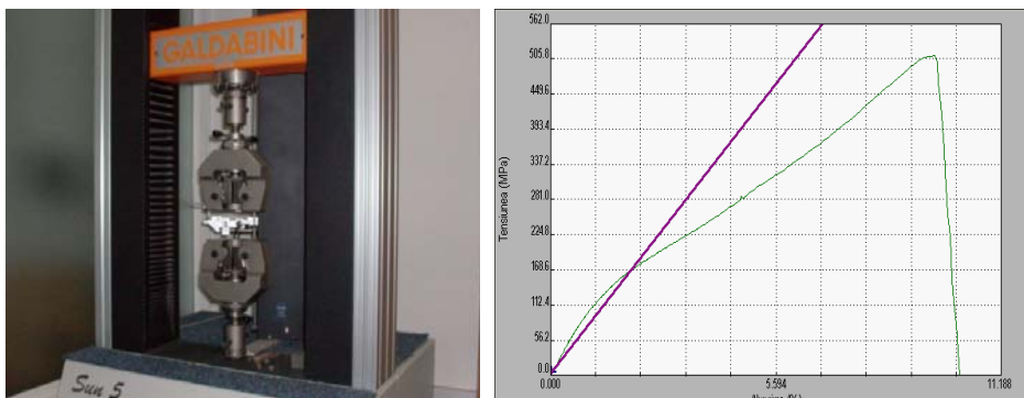
Figure 2. Testing the SLM samples on the Galdabini equipment from TUCN
