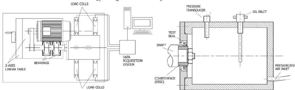
Figure 1. Schematic view of test system and test block
