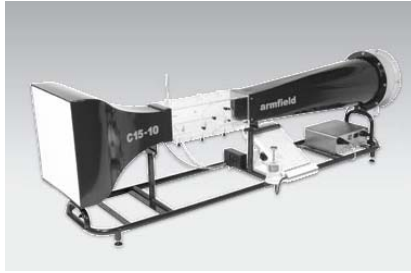
Figure 1. Wind tunnel ARMFIELD C15-10
