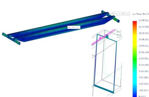
Figure 2. Von Mises stress for first model of crane
