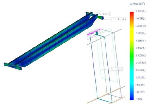
Figure 3. Von Mises stress for optimized model of crane
