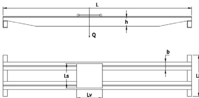
Figure 1. Basic geometry parameters of a crane with trolley
