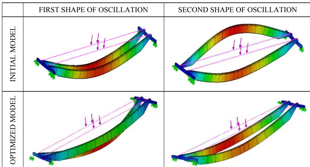
Figure 4. First and second shape of oscillation for two models of crane
