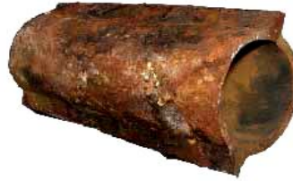
Figure 2. Sample of membrane tube baffle
