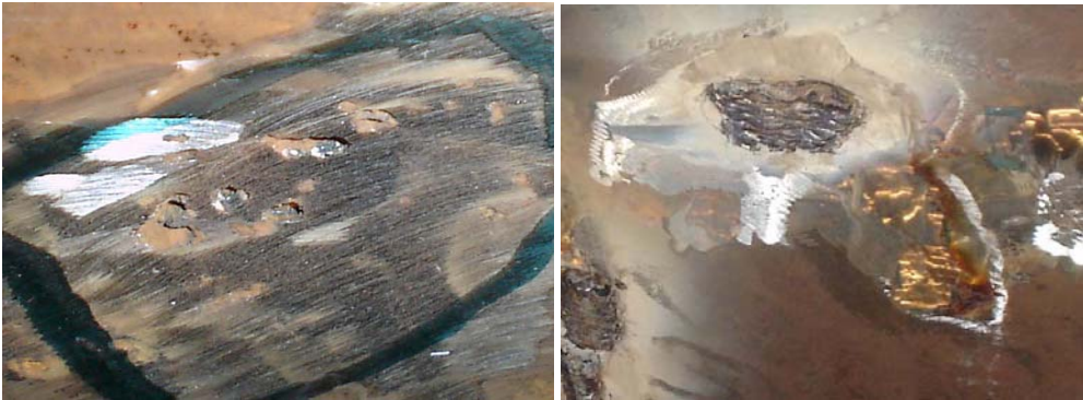
Figure 5. Marked areas with cavitations
