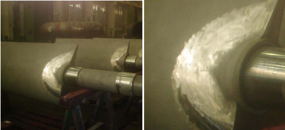
Figure 3. Cleaned and polished blades with marked places that has been the first priority for ultrasonic testing
