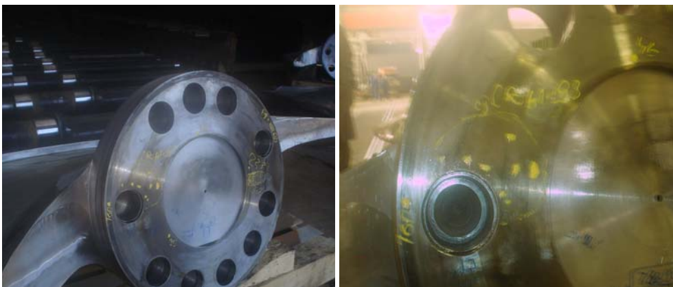
Figure 2. Shoulder blades of turbine with detected places with material non-homogeneity
