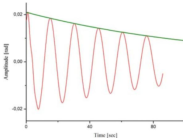
Figure 5. Amplitude interpolated by exponential decay function
