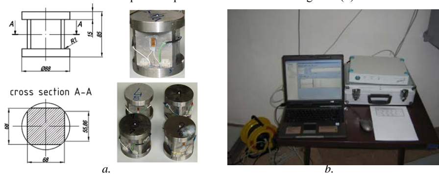
Figure 2. Total drawing force dynamometer (a) and "Spider 8" amplifying device (b)
