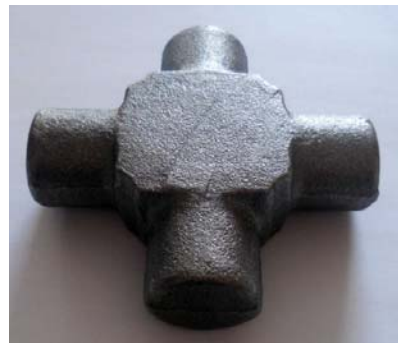
Figure 6. Cross joint part manufactured by orbital forging
