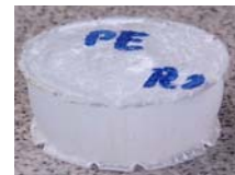
Figure 2. Specimens made from PA (left) and HDPE (left) after Rastegaev test
