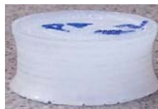
Figure 2. Specimens made from PA (left) and HDPE (left) after Rastegaev test
