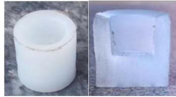
Figure 4. Specimens of PA after backward can extrusion
