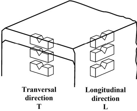
Figure 2. Cutting direction of specimen
