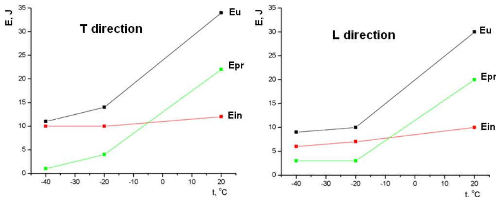
Figure 3. Dependence heat input vs. impact energies at all testing temperatures
