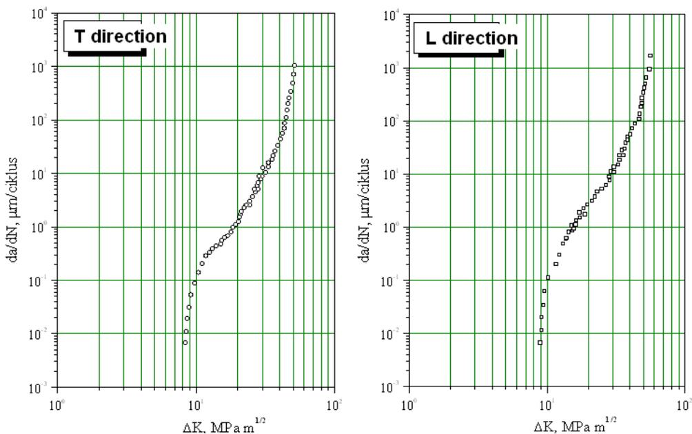
Figure 4. Diagram  $da/dN$  vs.  $\Delta K$  for T and L direction
