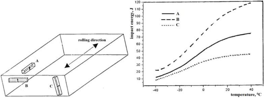
Figure 1. Influence of specimens direction on the impact energy
