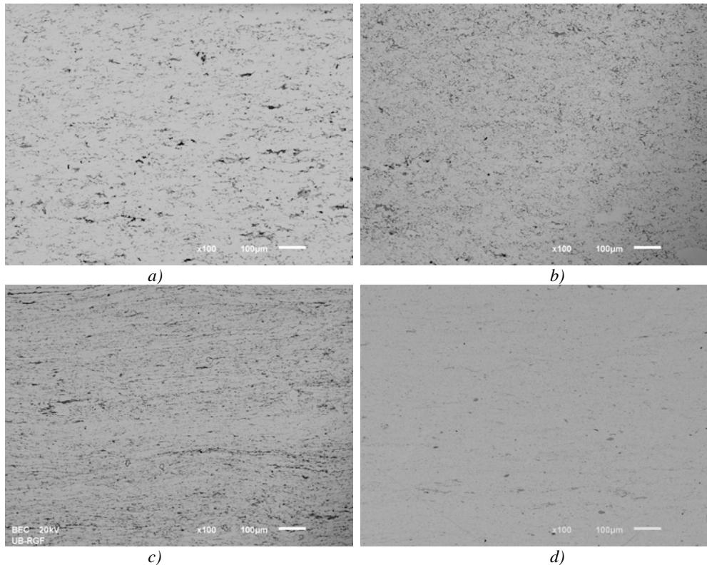
Figure 1. SEM images of microstructures of the obtained Ag-SnO<sub>2</sub> electrical contact materials
