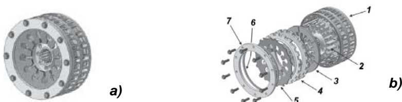
Figure 3. 3D explode view of an Formula 1 clutch a) assembly b) explode view 1)Clutch housing; 2)Hub; 3)Intermediate plate; 4)Clutch disc; 5)Diaphragm spring; 6)Pressure ring; 7)Cover
