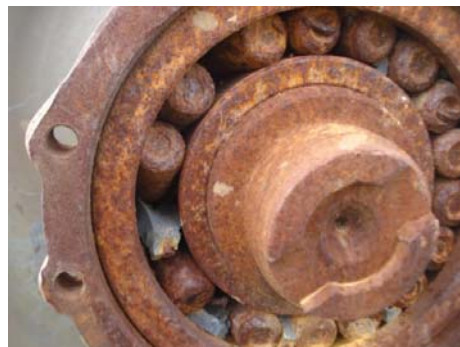
Figure 5. The consequences of lack of lubrication
