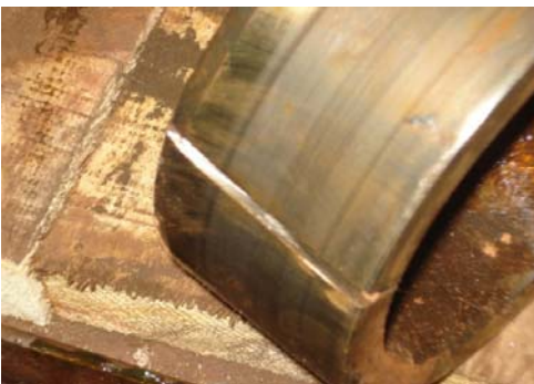
Figure 4. Cracks in the ring
