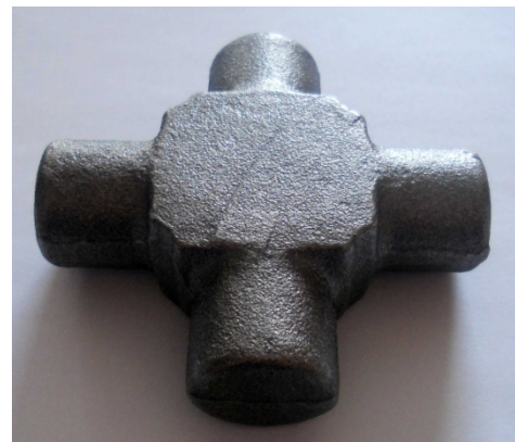
Figure 6. Cross joint part manufactured by orbital forging
