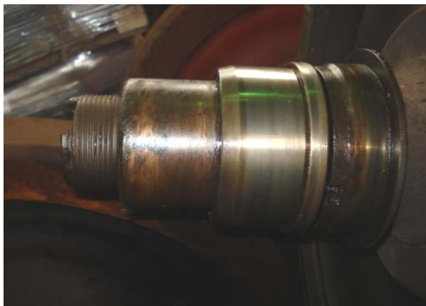
Figure 2. Damage deposit (sleeve), corrosion and etching Figure 3. The damaged surface and flaking
