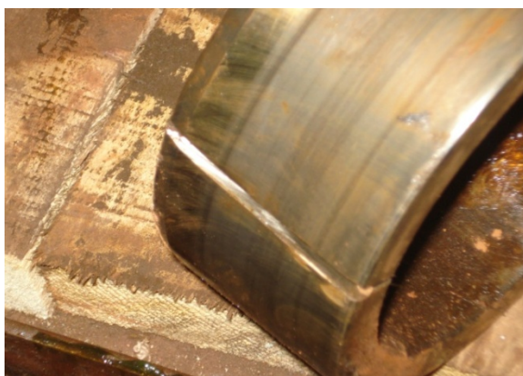
Figure 4. Cracks in the ring
