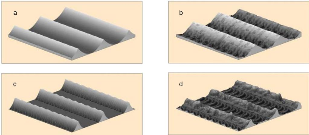
Figure 1. Surface topography for  $f=0.05 \text{ mm}\cdot\text{tooth}^{-1}\cdot\text{revolution}^{-1}$  and  $Rd=0.40 \text{ mm}$ , for  $E=0.001$ : a) simulated, b) experimental, and for  $E =0.100 \text{ mm}$ : c) simulated, d) experimental
