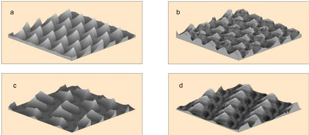
Figure 2. Surface topography for  $f=0.20 \text{ mm}\cdot\text{tooth}^{-1}\cdot\text{revolution}^{-1}$  and  $Rd=0.20 \text{ mm}$ , for  $E=0.001$ : a) simulated, b) experimental, and for  $E =0.100 \text{ mm}$ : c) simulated, d) experimental
