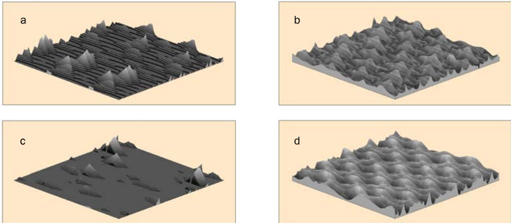
Figure 3. Surface topography for  $f=0.40 \text{ mm-tooth}^{-1} \cdot \text{revolution}^{-1}$  and  $Rd=0.05 \text{ mm}$ , for  $E=0.001$ : a) simulated, b) experimental, and for  $E =0.100 \text{ mm}$ : c) simulated, d) experimental
