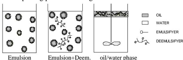
Figure 1. Mechanisms of emulsion splitting by INA-Deemulzin
