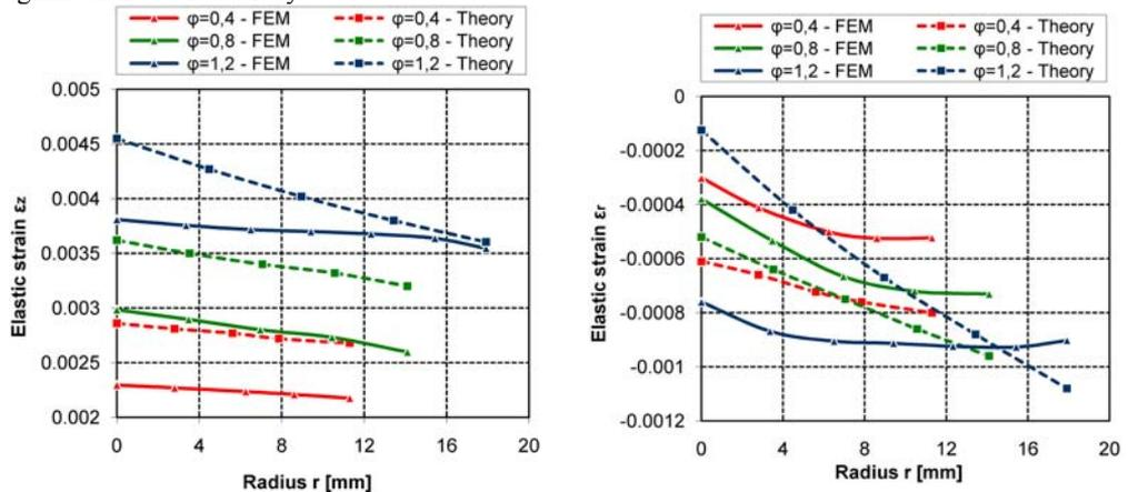
Figure 1. Engineering (elastic) strains in axial (left) and radial (right) direction
