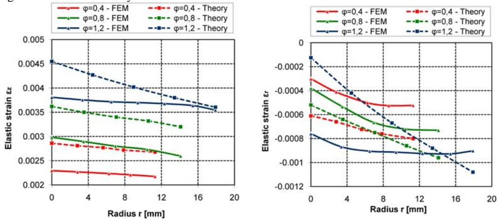
Figure 1. Engineering (elastic) strains in axial (left) and radial (right) direction
