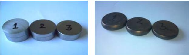
Figure 2. Test parts for compression test before, (left) and after deformation, (right)
