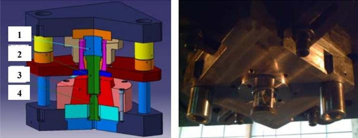
Figure 3. 3D model of the experimental tool with load cell -1, punch -2, die -3 and ejector -4, (left) and experimental tool with load cell mounted in the housing, (right)
