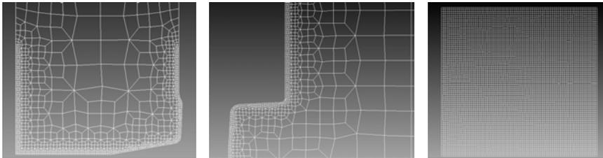
Figure 4: Punch and die meshes a) and initial mesh of the workpiece b)
