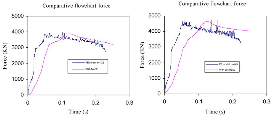
Figure 3. punch force – time curves, experiment vs. prediction with  $m=0,3$  and MoS2 a) and with  $m=0,5$  and without MoS2 lubricant
