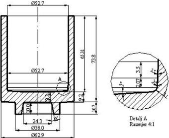
Figure 1. Geometry of workpeace after combined extrusion
