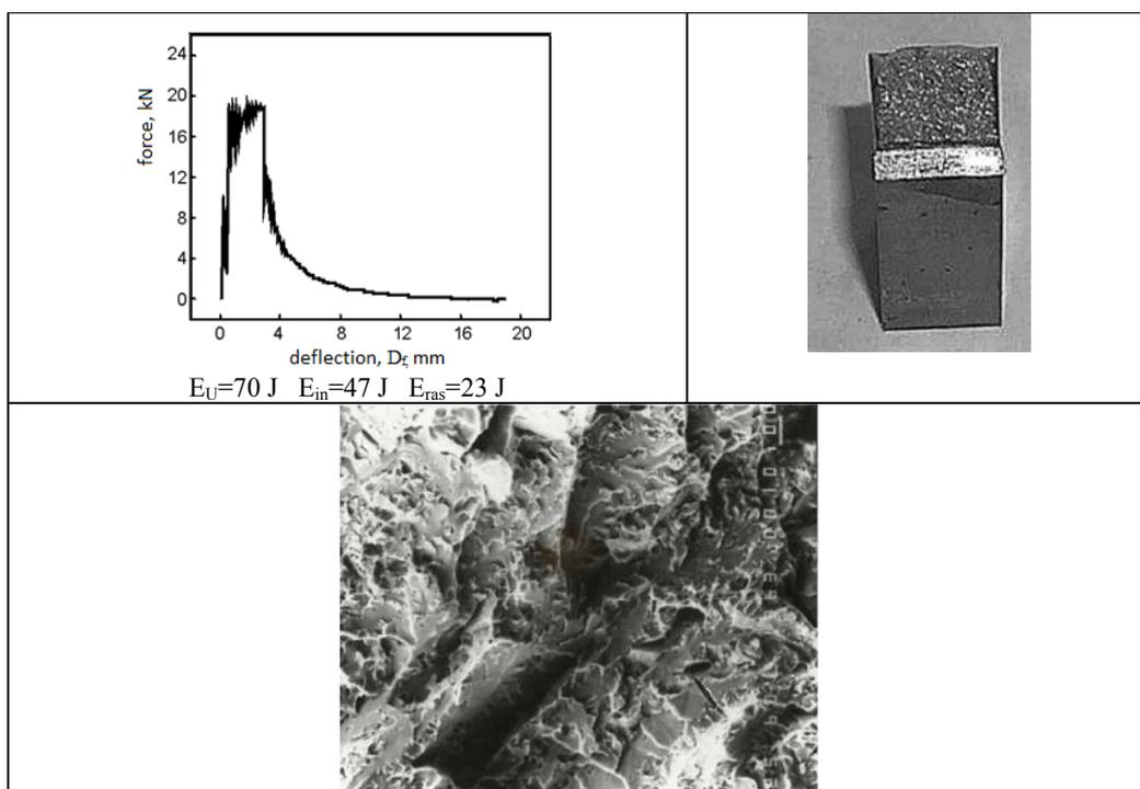
Figure 3. Fracture analysis at  $-55^{\circ}\text{C}$ : a) diagram  $F\text{-}D_f$ ; b) fracture surface of Charpy specimen; c) fractography- brittle intergranular fracture at lower temperature
