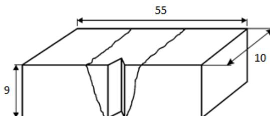
Figure 1. Sketch of Charpy specimen with V notch in weld metal
