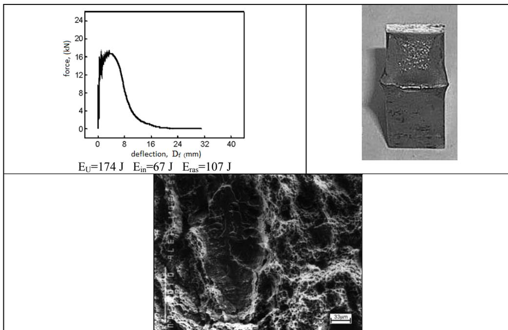
Figure 2. Fracture analysis at  $20^{\circ}\text{C}$ : a) diagram  $F\text{-}D_f$ ; b) fracture surface of Charpy specimen; c) fractography- mixture fracture; ductile and brittle fracture at room temperature
