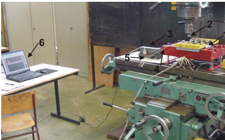
Figure 6. Connected information measurement system for temperature measurement: 1 - work piece, 2 - tool for FSW, 3 - measuring module, 4 - thermo couples, 5 - connection terminals and 6 - PC computer [5]
