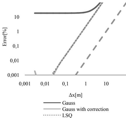
Figure 6. Discretization error on non-orthogonal grid
