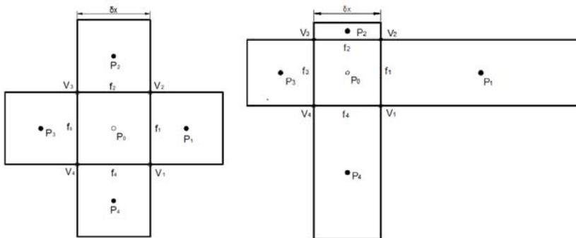
Figure 1. Cartesian (left) and orthogonal non-uniform numerical grid (right)
