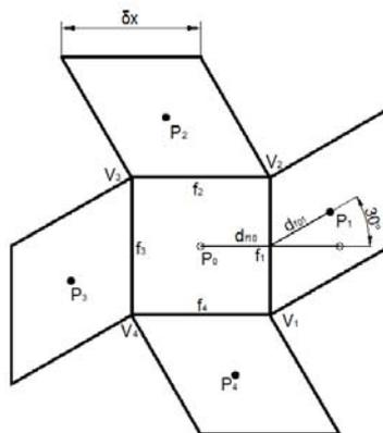
Figure 2. Non-orthogonal numerical grid
