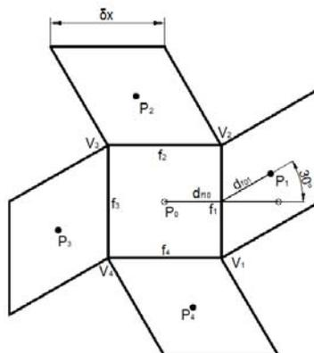
Figure 2. Non-orthogonal numerical grid
