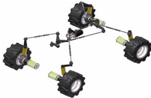
Figure 4: Connection of the spatial leverage mechanism for controlling direction of the mobile platform and the wheels.
