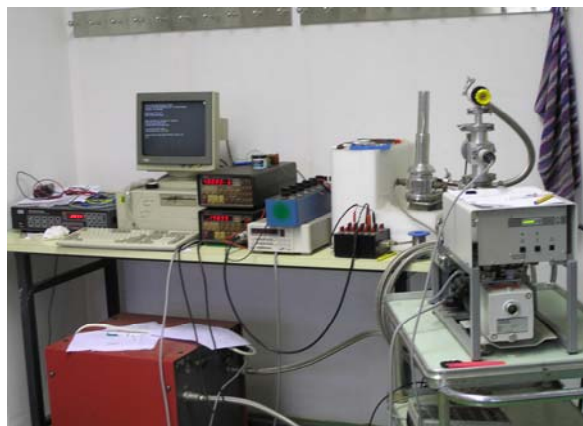
Figure 1. Measuring system used to determine the conductivity
