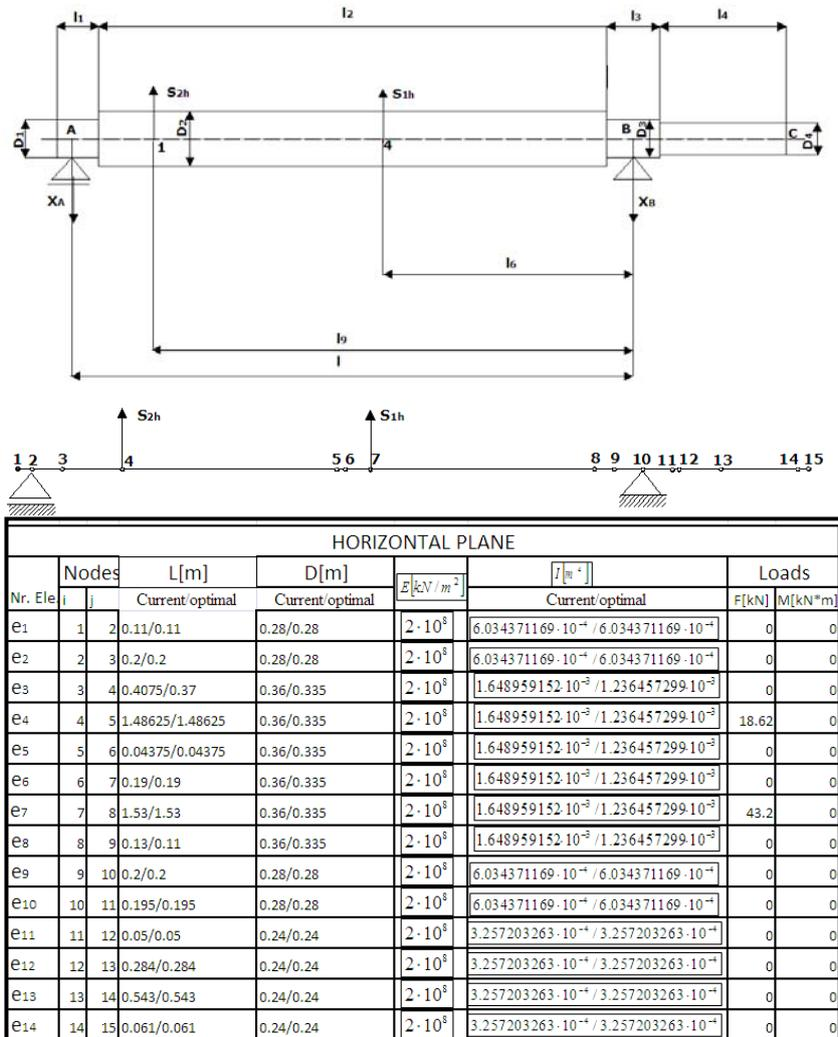
Figure 1. Mechanical and FE model with respective data-horizontal plane
