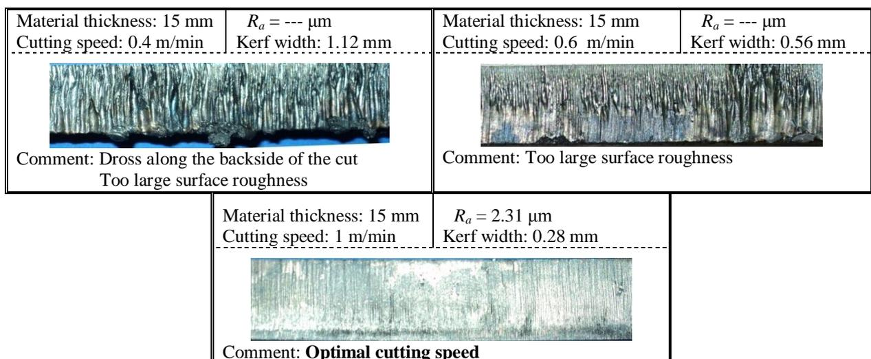
*Figure 4. The photographs of cut samples – material thickness of 15 mm*
