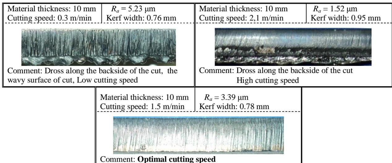
Figure 3. The photographs of cut samples – material thickness of 10 mm
