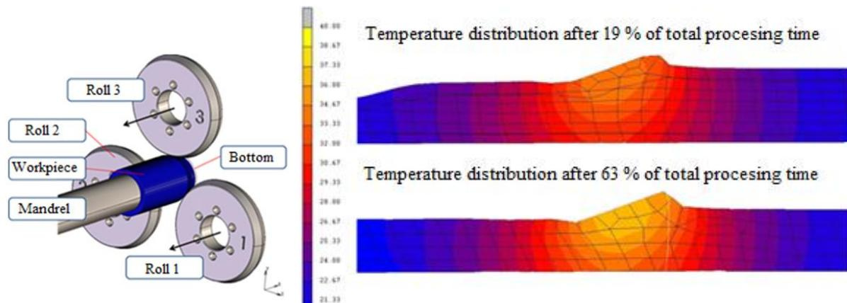
Slika 3. CAD model and temperature distribution in deformation zone obtained from FEM process simulation
