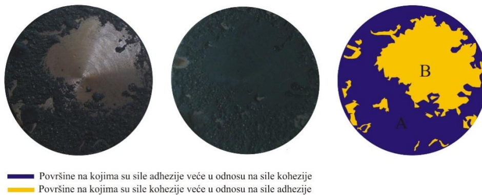
Figure 1. Dominant forces on the fractured surface of the experimental samples
