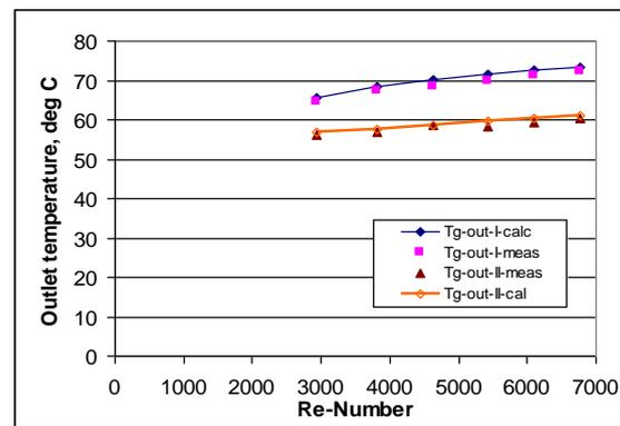
Figure 6. Experimental and numerical outlet gas temperature
