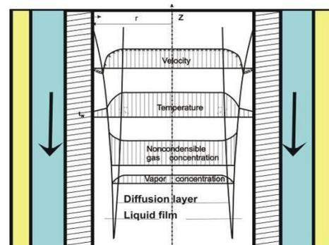
Figure 2. Physical model of experimental cases
