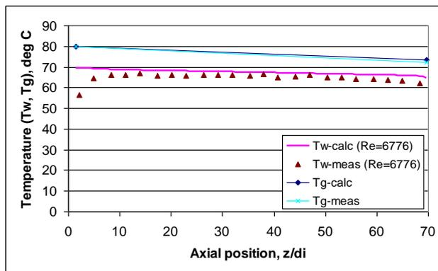
Figure 5. Experimental and numerical wall and gas temperature,  $Re=6776$
