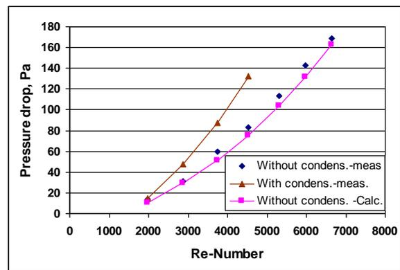
Figure 4. Pressure drop in the conduit with and without condensation
