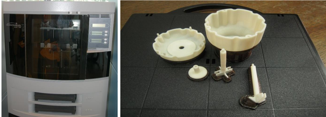
Figure 9: Rapid prototyping system based on FDM technology (Dimension Elite) and processed functional parts on working platform
