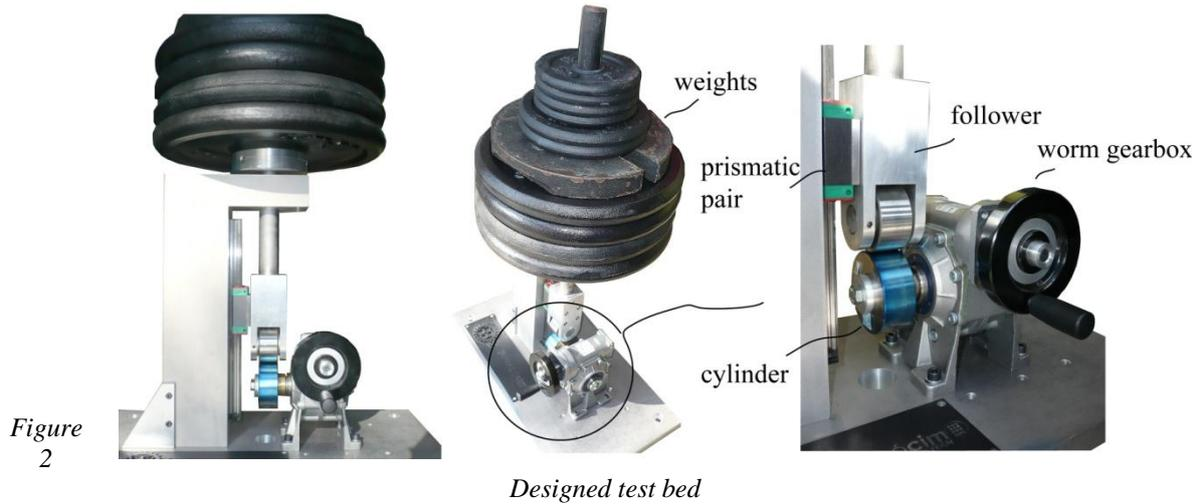
The analyzed contact case is between a crowned roller and grinded cylinder. A cam locally in each contact point is approximated to a cylinder with the radius the local curvature radius  $r_c(q)$  of the profile as it is seen in Figure 1b. In Table 1 are presented the surface roughness, geometrical and material properties of the crowned roller and the grinded cylinder.
