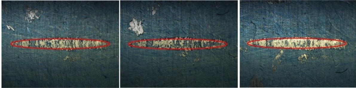
Figure 3 Experimental contact ellipse when  $F=790,8\text{ N}$
