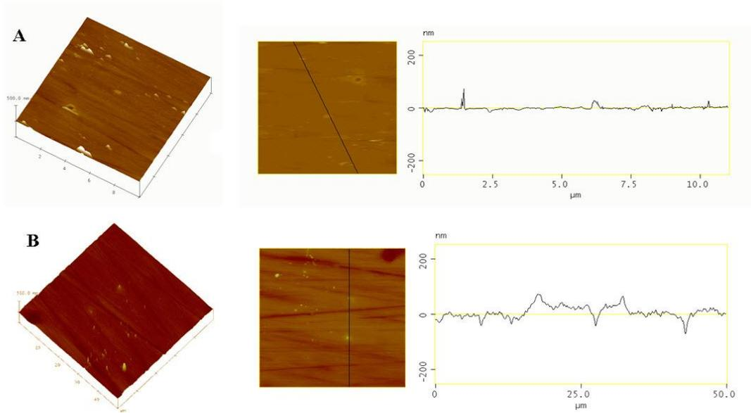
Figure 1. AFM analysis of deposited  $\text{TiO}_2\text{-ZrO}_2$  films calcined at  $401\text{ }^\circ\text{C}$ ; 3D image and AFM profile (A)  $10\text{ }\mu\text{m} \times 10\text{ }\mu\text{m}$  scan size and (B)  $50\text{ }\mu\text{m} \times 50\text{ }\mu\text{m}$  scan size
