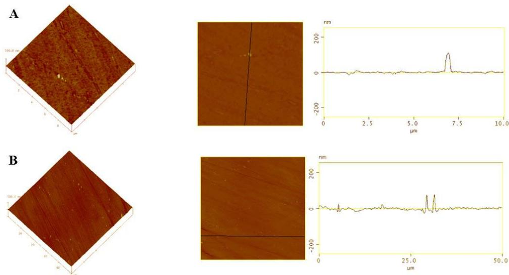
Figure 2. AFM analysis of deposited  $\text{TiO}_2\text{-ZrO}_2$  films calcined at  $600\text{ }^\circ\text{C}$ ; 3D image and AFM profile (A)  $10\text{ }\mu\text{m} \times 10\text{ }\mu\text{m}$  scan size and (B)  $50\text{ }\mu\text{m} \times 50\text{ }\mu\text{m}$  scan size
