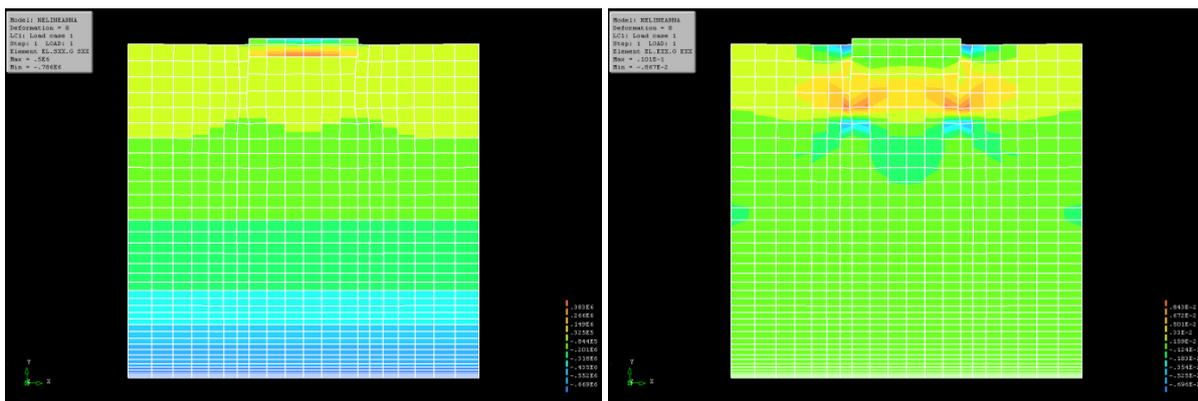
Figure 4. Stress and dilatation response of the foundation and soil after dynamic loading
