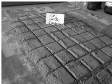
Figure 1. Composite sample of flotation tailings prepared for experimental testing
