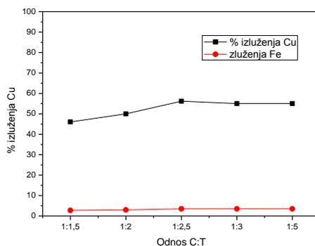
Figure 4 Dependence of the copper leaching degree on relation solid:liquid at pH=1, temperature: 80°C, time: 4 h
