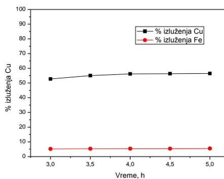
Figure 3. Dependence of the copper leaching degree on leaching time in relation S:L = 1:2.5, pH = 1, temperature: 80°C
