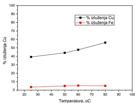
Figure 2. Dependence of copper leaching degree on temperature in relation S:L = 1:2.5, pH = 1, time: 4h
