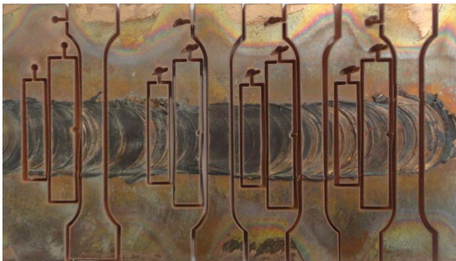
Figure 2. Showing excised samples of welded workpieces for copper alloys
