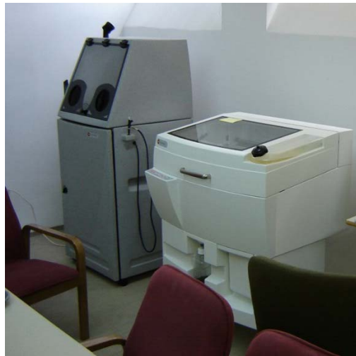
Figure 1. ZCorp printer which made the parts for the research
