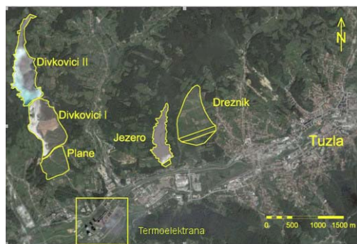
Figure 1. Disposition of slag and ash deposition sites of TPP Tuzla (source-Google Earth)
