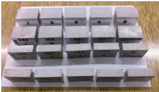
Figure 1. The samples with linear cuts prepared for the measurement of surface roughness (left), and the measurement of surface roughness (right).
