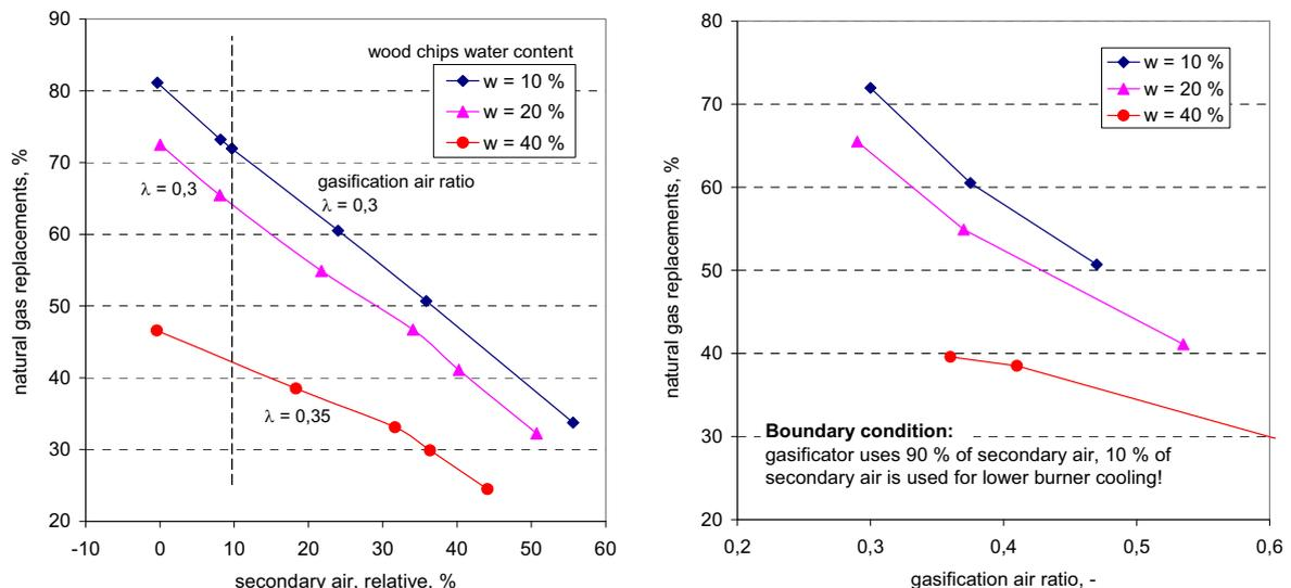
Figure 2. Impact of wood chips water content and gasification air ratio on natural gas replacements at lower burners
