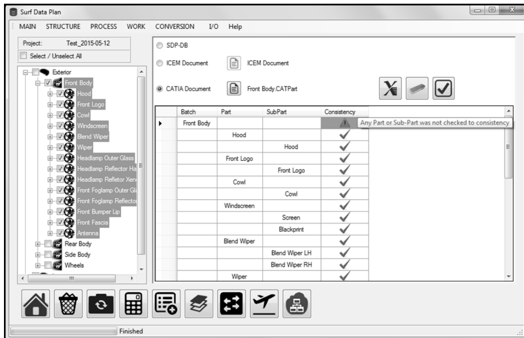
Figure 3. KBD application prototype for automotive styling checking the consistency using RDBMS.
