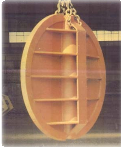
Figure 1. Butterfly pre-turbine valve gate on HE "Glava Zete"
