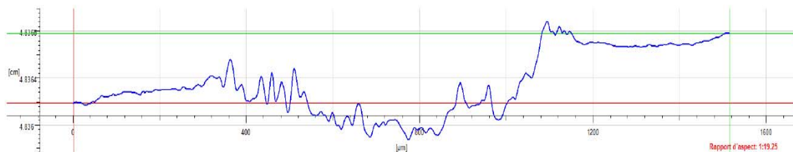
Figure 6. Indentation profile for F = 450\text{ N} , n = 5 and the ultrasonic-vibrations-assisted process.
