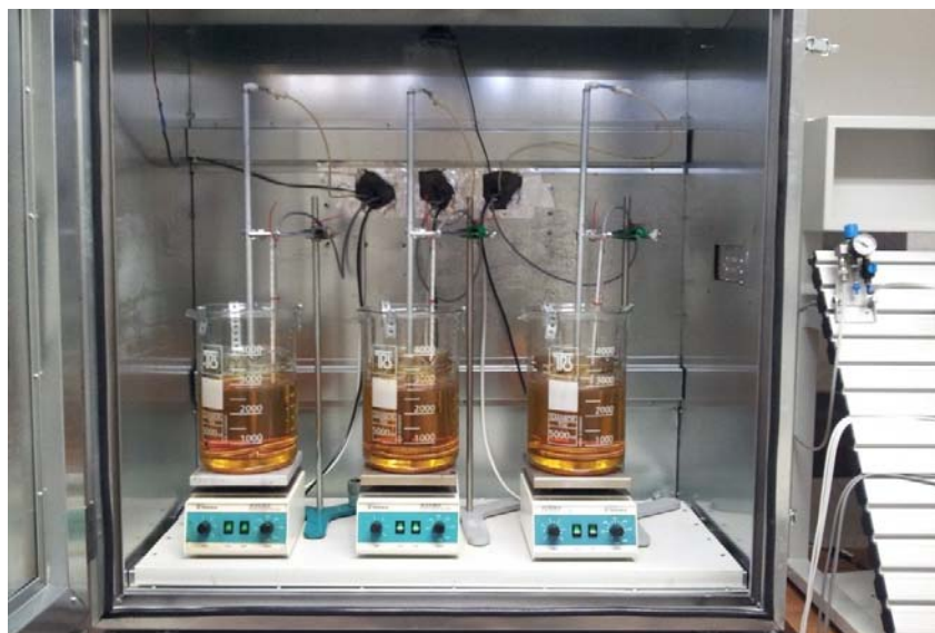
Figure 2. Preparation of implemented dry thermal test for accelerated oil ageing.
