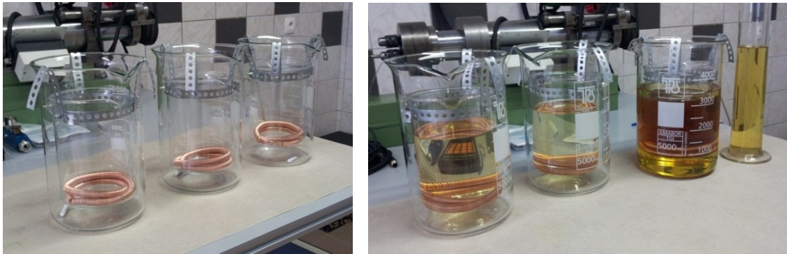
Figure 1. Preparation of glassware and copper wire for implementation of the test (left) and preparation of the samples (right).
