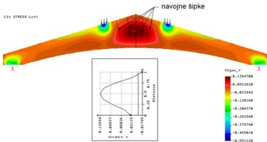
Figure 7. Stress state of transverse stresses in the gable-beam
