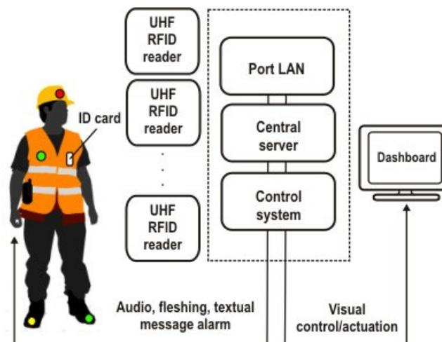
Figure 1. Scheme of the PPE-RFID solution proposed for the Port of Bar [15]
