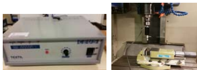
Figure 5. Left: external vibrations generator. Right: burnishing tool attached to milling machine.
