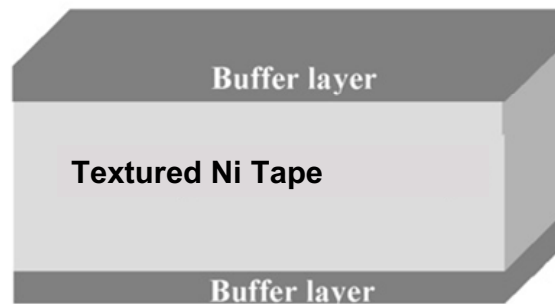
Figure 1. Schematics representation of YSZ/Ni buffer layer structure.
